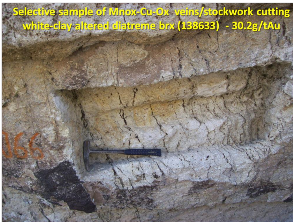
Figure 26. Au-bearing Mn-oxide/carbonate -only narrow veinlets cutting clay -altered diatreme – Cerro Hermoso . Teck sample with assay results.
