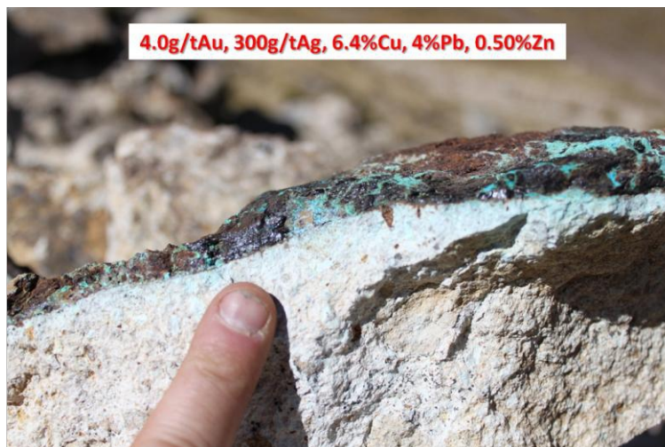
Figure 23. Cu/Fe/Mn -oxide only narrow veinlets cutting clay -altered diatreme – Cerro Hemoso . Teck sample with assay results.
